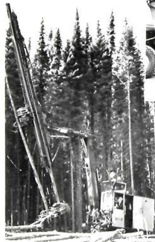
◊ A full-tree harvester shears off, at ground level, trees up to 22" in diameter.
